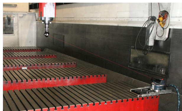
THE INTERFEROMETER OF THE LASERTRACER FOLLOWS THE REFLECTOR ATTACHED TO THE SPINDLE AUTOMATICALLY THROUGH THE WHOLE VOLUME. DURING THIS PROCESS, HIGHLY ACCURATE MEASUREMENTS ARE CARRIED OUT, FROM WHICH THE DEVIATIONS WILL BE CALCULATED.
