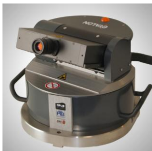
THE LASERTRACER IN COMBINATION WITH A REFLECTOR IS THE ONLY NECESSARY MEASUREMENT EQUIPMENT.
