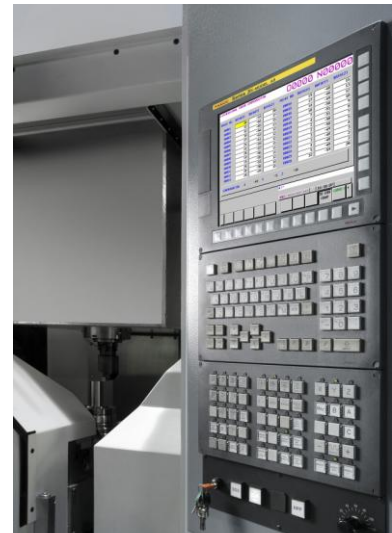
THE FUNCTION „3D ERROR COMPENSATION“ FOR THE FANUC CNC CONTROLLERS OF THE SERIES 30I AND 31I-A5 CORRECTS GEOMETRIC MACHINE ERRORS.
