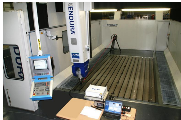
figure 1: FOOKE ENDURA 905 Linear during the volumetric calibration
