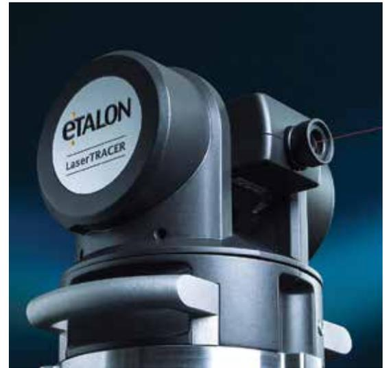
machine tools. It automatically tracks a reflector, and so allows for the high precision identification of geometrical deviations. A key feature is that it gives extremely high accuracy of the centre of rotation thanks to a patented measurement technique: a sphere with a form deviation of just 50 nanometers is used as an optical reference for the interferometer. As a consequence, the mechanical errors of the rotation and swivel axes are fully compensated.
