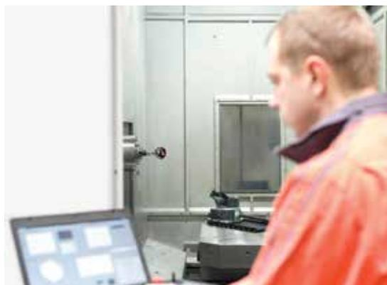
The required NC programs are automatically generated by Etalon's software, and the respective distances to the tool centre point determined via interferometer. The Etalon system transfers the recorded measured data to the connected Trac-Cal measuring software, which automatically processes the measured data. The compensation data obtained such can be visualised and then directly imported into the control software of the machine tool.
